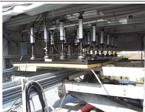
Picture 4 24 suction cups evenly distributed over the collector surface. Positive and negative forces applied up to 3250 Pa. On the picture uplifting force of 3200 Pa is shown. No problems observed
